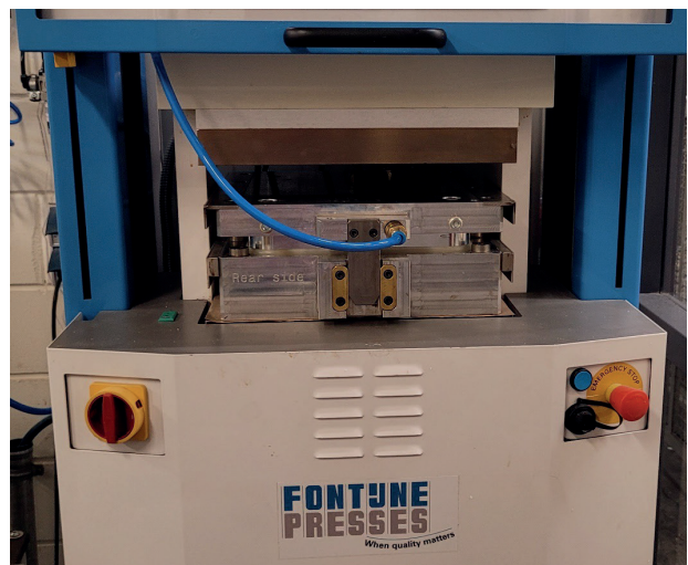
Picture 3: Lanulfi mould in the Fontijne press ready to be heated and put under pressure. The blue vacuum line is also attached.
