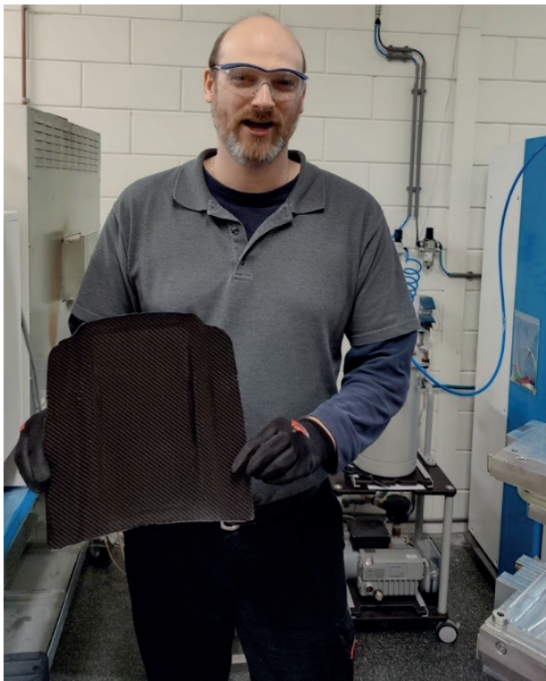
Picture 1: Application engineer Ward Steijn showing the first result of a thermopress cycle with snap-cure carbon fibre prepreg and Teccore TG180. Cycle time 7 minutes.
